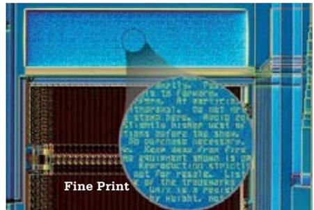
print in the world. HP wrote phrases like 'not for resale' on chips with letters just six microns tall – that's six-thousandths of a millimeter. The chips were used inside oscilloscopes during the 90s. You can find more of these kind of tiny silicon pictures on [micro.magnet.fsu.edu/creatures](http://micro.magnet.fsu.edu/creatures).
